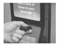
Note: If the right light on the fob illuminates, move the fob slightly to re-align it with the infrared window on the door. Once re-aligned, the right light will turn off while the left light should remain lit. If both lights turn off then the fob requires re-activation by pressing the activation button.
