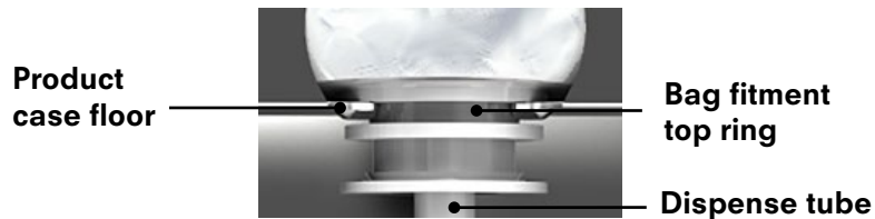
Figure 9: Dairy bag fitment secured on product case floor
