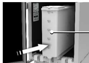
Figure 43: Install tank into dispenser
