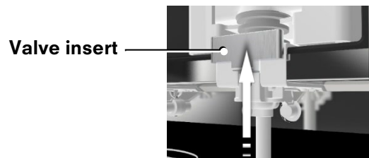
Figure 32: Reinstall the valve insert
