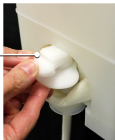
Figure 37: Shorten stopper and lock into place
