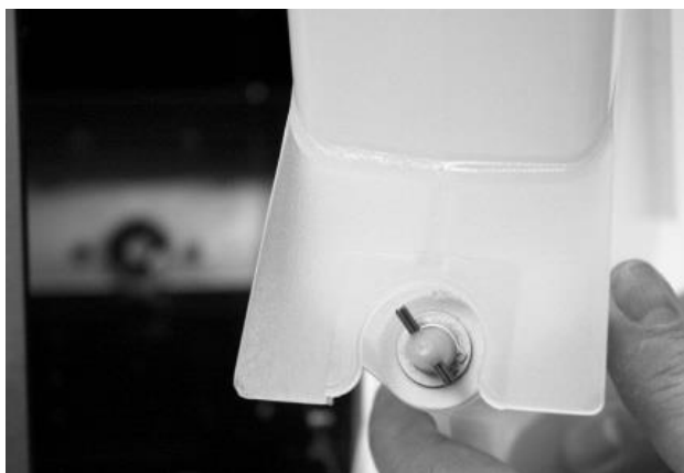
Figure 7: Drive pin on the auger assembly at the back of the hopper
