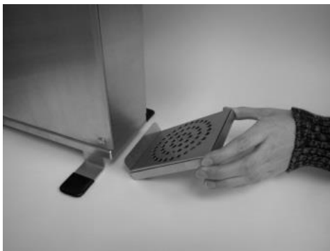
Figure 12: Removing the catch tray
